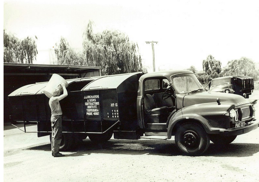
Garbage Cupboard Wagon 1962. It wasn't until 1968 that the first garbage compactor collection vehicle was designed & built. (Photo: courtesy Idwall Richards)
