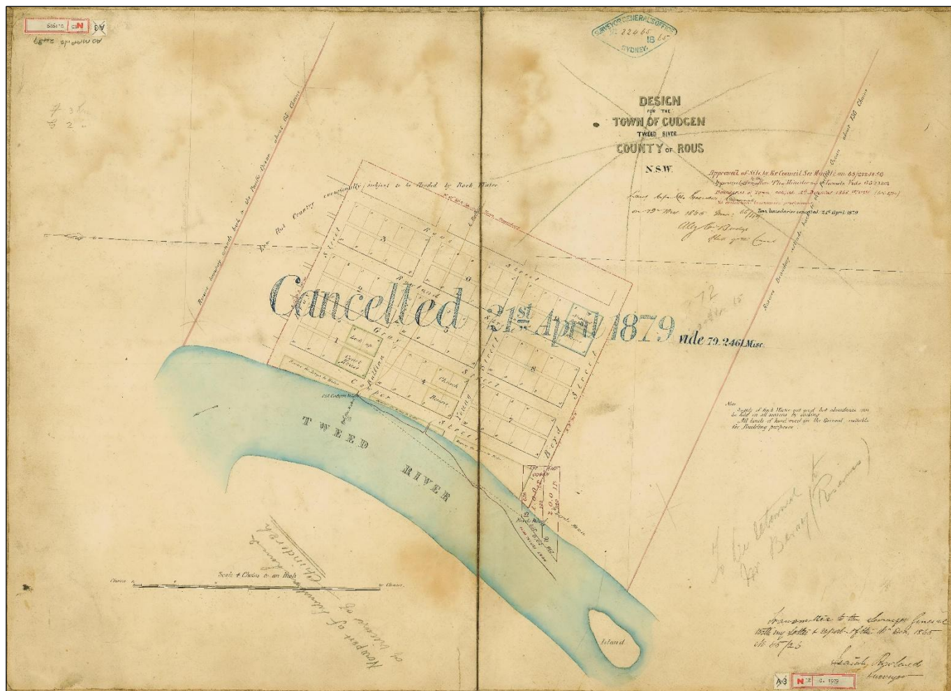
Figure 7. The first ever plan of subdivision for Cudgen (now Chinderah) – drawn by Isaiah Rowland in 1865. It was the first plan for a town in the Tweed. It has a number of errors, some of which were corrected on this original, presumably at head office in Sydney. For instance: the position of the shoreline in relation to the blazed tree on the foreshore (the correction is marked with a black solid line within the river); and the angle of the reserve boundaries which Rowland drew parallel to the boundaries of the town (the red lines to the far left and right). The reserve boundaries should have been drawn at right angles to the (magnetic) north arrow. Crosses in pencil have been drawn through the incorrect reserve boundary lines, and the correct position of the lines has been drawn in faint pencil. Also, in this plan Rowland said the tree blazed broad arrow over Ill was an 'Apple Tree'. In his plan of the lower reaches of the Tweed River of 1863, he said the same tree was a 'Tea Tree'. The first freehold lots purchased in Chinderah township (by Thomas Boyd) have also been added to this plan a number of years after it was drawn (on the right hand side of the township and partly in what was marked-up as river by Rowland). These lots were surveyed by Frederic Verdon Hunter for a plan he made in 1877, and they convey the extent to which the position of the foreshore was marked in error by Rowland. This town plan was cancelled before any of the portrayed lots were sold. Presumably some number of people continued to illegally occupy this crown land well after 1865-66. Thomas Boyd selected two lots of 40 acres about 1.5 km upstream in 1868, so possibly could have avoided illegal occupation of crown land by moving house to there. It was not until sometime after 1877 when he purchased the two lots in Cudgen Village that at least some of his enterprise there was no longer on crown land. Three street names on the plan memorialise arguably the three chief men of the Tweed at the time – Samuel Gray, Joshua Bray and Thomas Boyd. Two other streets are named after the Premier of NSW at the time, Charles Cowper, and surveyor Rowland himself.
